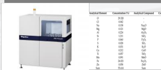
Model: Rigaku XRF Purpose: Material Analysis
